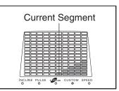
tings are not shown in the matrix.) The speed settings for the next several segments will be shown in the columns to the right.
